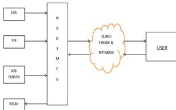
*Figure 7 | Block diagram for implementation*
